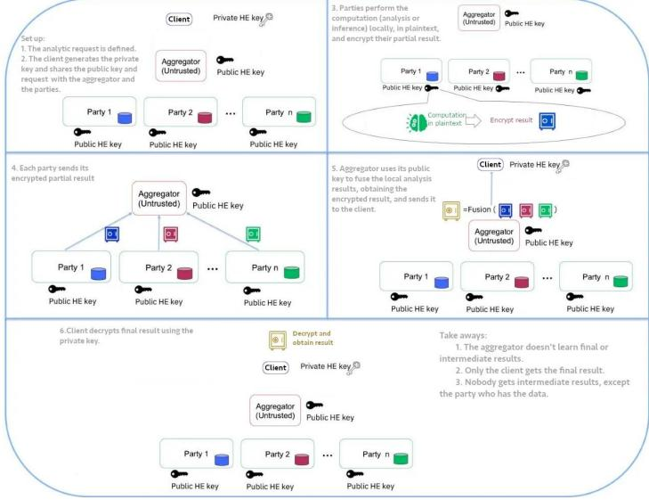
Diagram of analysis and inference scheme for machine learning models using homomorphic encryption, adapted from [4].
