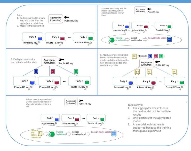
Diagram of training scheme for machine learning models using homomorphic encryption [4].
